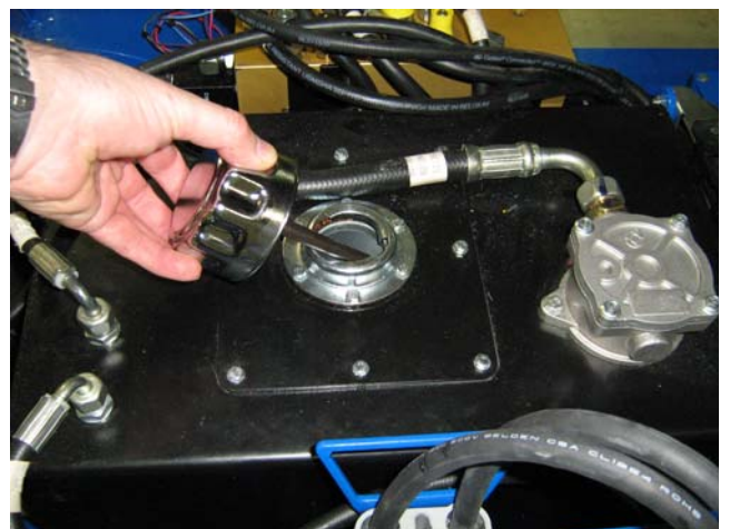
Figure 3-25: Hydraulic Tank Dip Stick
