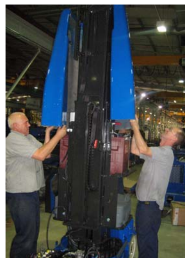
Figure 3-8: Mast Cover Removal
