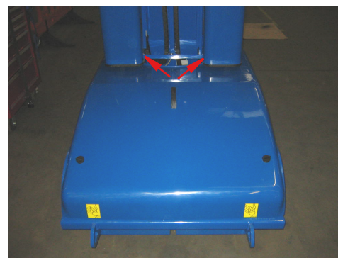
Figure 3-8: Mast Cover Removal
