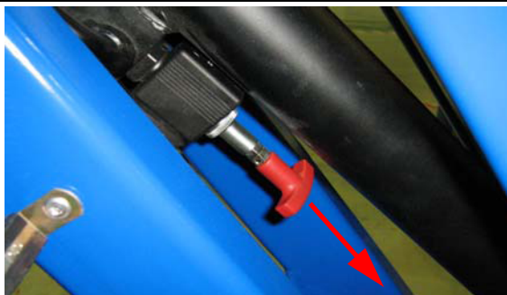
Figure 9: Emergency Lowering - Jib Valve
