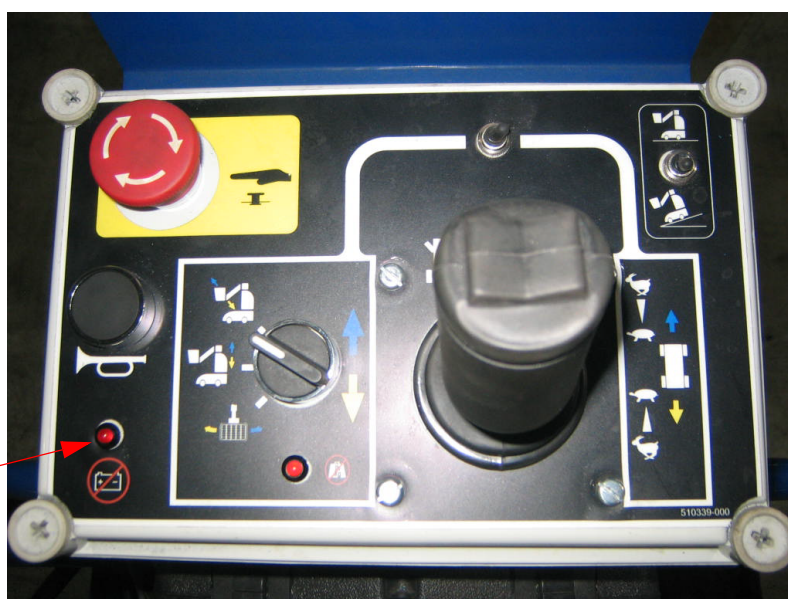
Figure 3-30: Upper Control Panel with Battery Indicator
