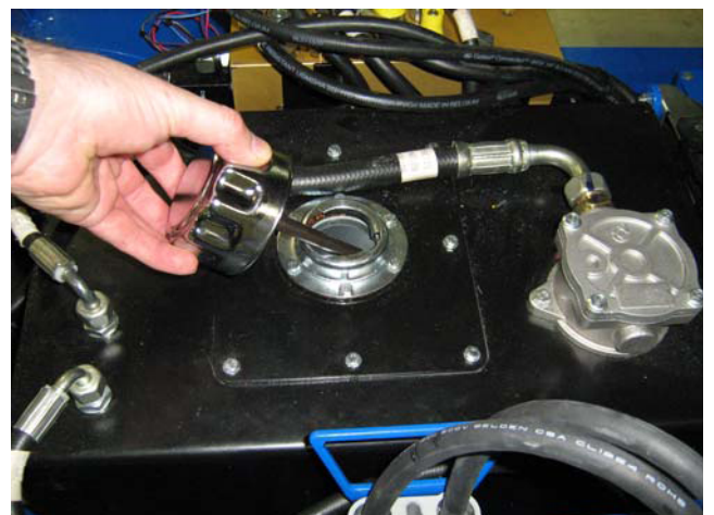
Figure 3-25: Hydraulic Tank Dip Stick
