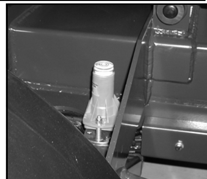
Figure 3-3: Level Sensor
