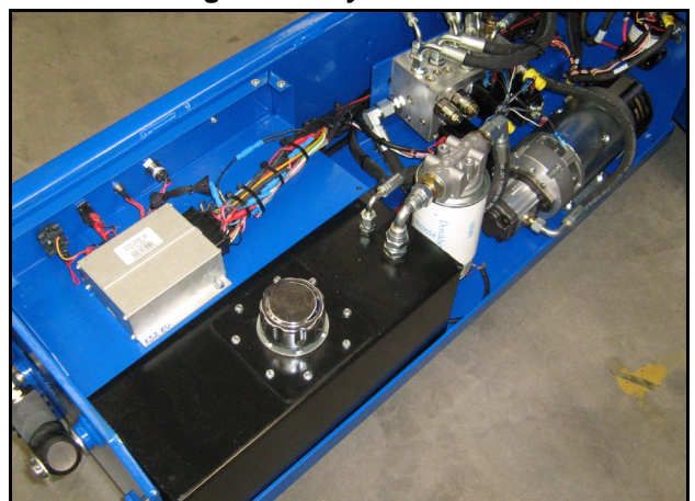
Figure 11: Hydraulic Fluid Reservoir
