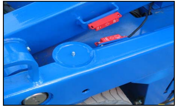
Figure 3-6: Proximity Switch
