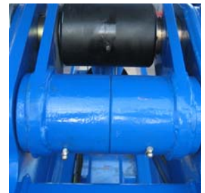
Figure 3-4: Lift Ram & Scissor Pin Lubrication Points
