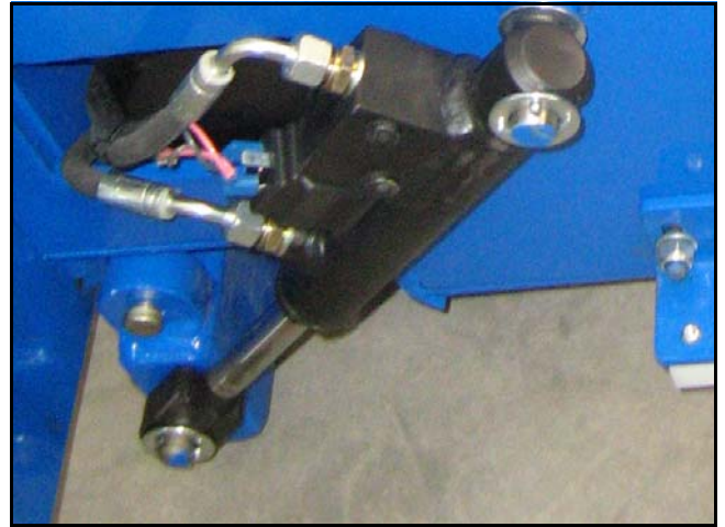
Figure 3-14: Depression Cylinder
